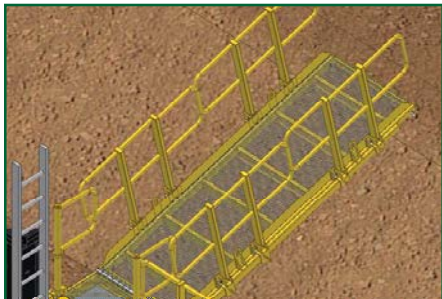
Steel Manbridge w- Guard Rail
